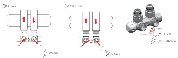
In order to change configuration of the valve from monotube to bitube close the by-pass using 6 mm Allen key rotating it in vertical direction as shown in the picture. Open the by-pass in order to make monotube configuration.
