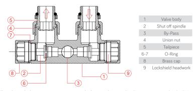
All technical characteristics are provided according to the European standard EN 215 "Thermostatic radiator valves. Requirements and test methods". Threads are in compliance with EN-ISO 228/1 standard.
